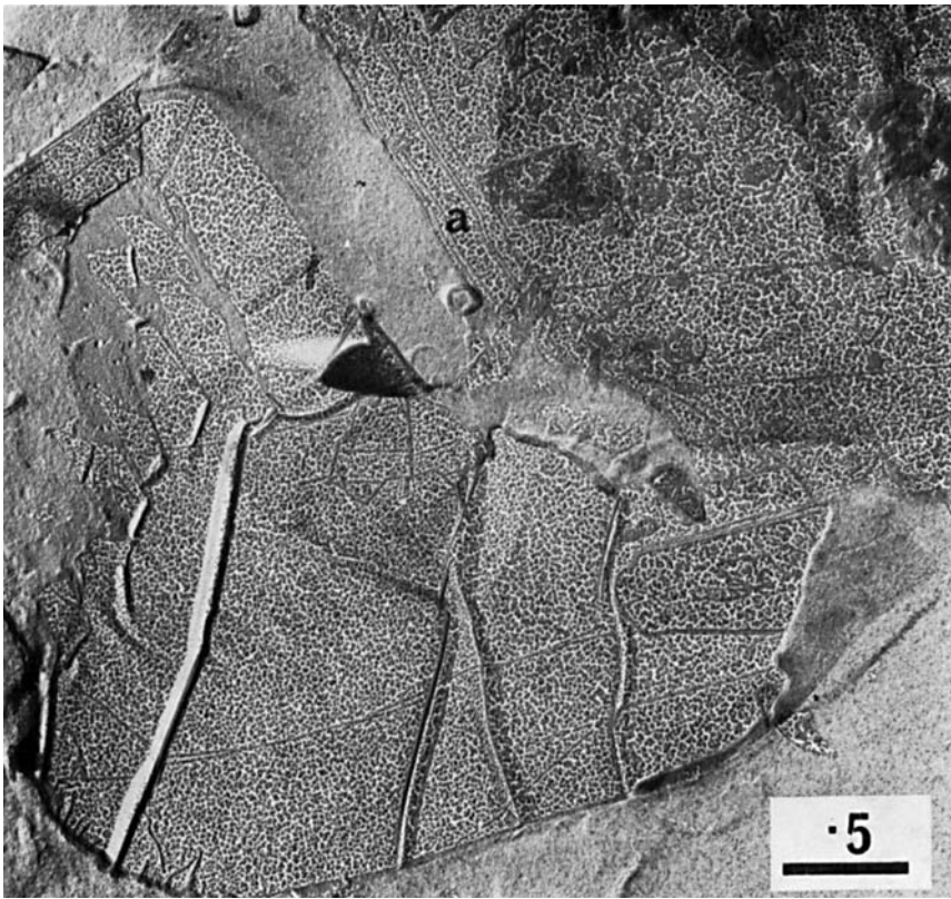
FIG. 1 Typical decoration pattern on a particle of natural talc. Numerous crystal lattice planes are shown (a). ( \times 30\ 000 ) Scale refers to 1.0\ \mu .
