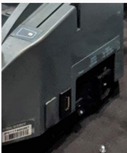
Picture: Externally exposed USB port on the side of the Electronic Pollbook Stand. The port does not get locked when the stand is locked and it does not have a lid or hook on which to place a seal.
